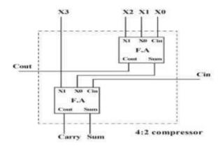
Convential 4-2 compressor system is shown in Figure 2.
